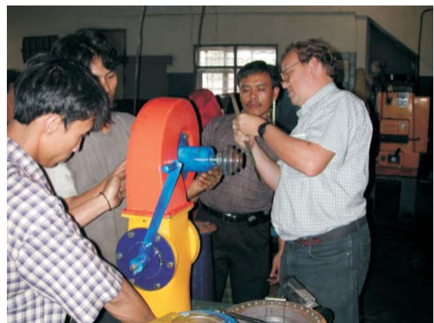
Photo 4: Technicians from CIT with assistance from MHPP are currently developing a range of pico-hydro turbines suitable for small power requirements
